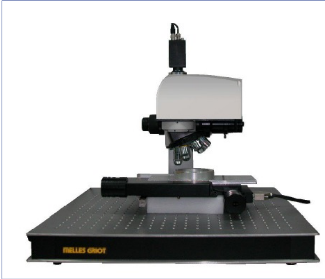
Fig 2.4. Non-contact confocal microscope used for profilometry measurements (Plm, Sensofar, Terrassa, Barcelona, Spain).
